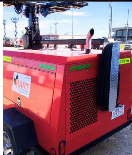
Above shows one running light tower with the remote units using 110v cord plug-ins, this eliminates two running motors in this configuration.
