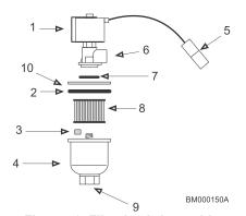
Figure 49. Filter Lock Assembly
