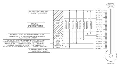
Figure 46. Engine Operating Temperature Specifications - Deutz - Sheet 1 of 2
