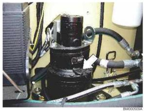
Lube Point(s) - Level/Fill Plug Capacity - 43 oz (1.3 L) Lube - 90w80 Gear Oil
