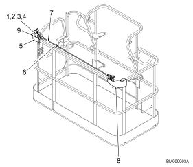
Figure 21. Bolt-On External Fall Arrest System
