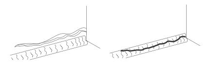
Figure 1. Parent Metal Crack
