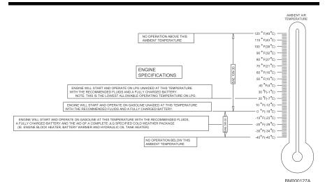
Figure 44. Hydraulic System Operating Temperature Specifications — Sheet 1 of 2
