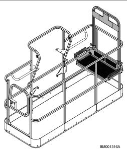
Figure 30. Boom Platform Deck
