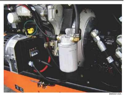
Lube Point(s) - Replaceable Element Interval - Change in accordance with engine manual
