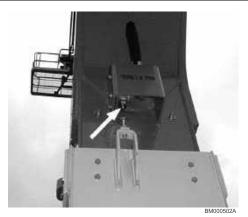
Figure 4. Tower Boom Horizontal Limit Switch
