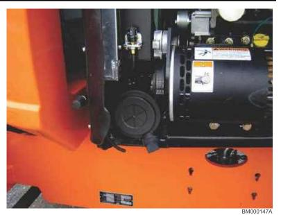
Lube Point(s) - Replaceable Element Interval - Every 6 months or 300 hr of operation or as indicated by the condition indicator
