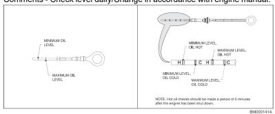
Figure 48. Deutz 2011 Engine Dipstick
