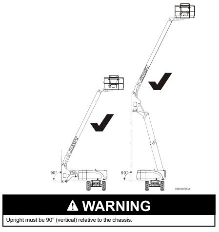
Figure 5. Boom Upright Positioning - Correct
