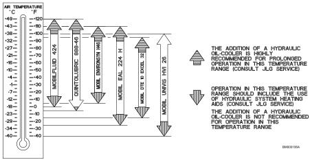
Figure 43. Hydraulic System Operating Temperature Specifications
