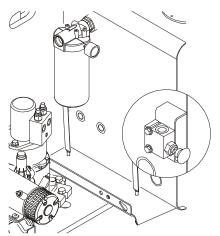
Figure 14. Re-leveling Valve
