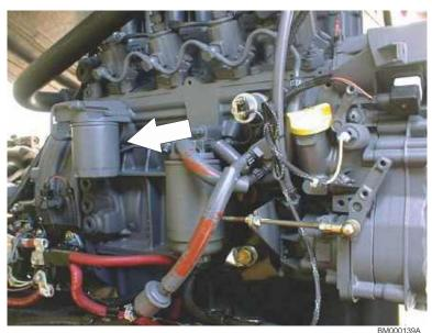
Lube Point(s) - Fill Cap/Spin-on Element
