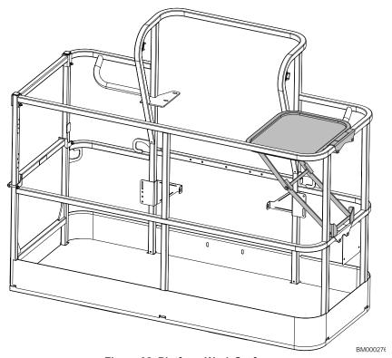
Figure 32. Platform Work Surface
