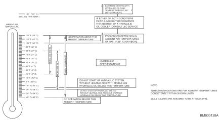
Figure 45. Hydraulic System Operating Temperature Specifications — Sheet 2 of 2
