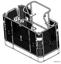
Figure 28. Platform Mesh to Mid Rail
