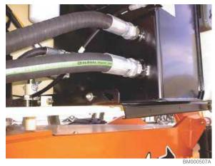
Lube Point(s) - 2 Grease Fittings Capacity - A/R Lube - MPG Interval - Every 3 months or 150 hr of operation Comments - Remote Access
